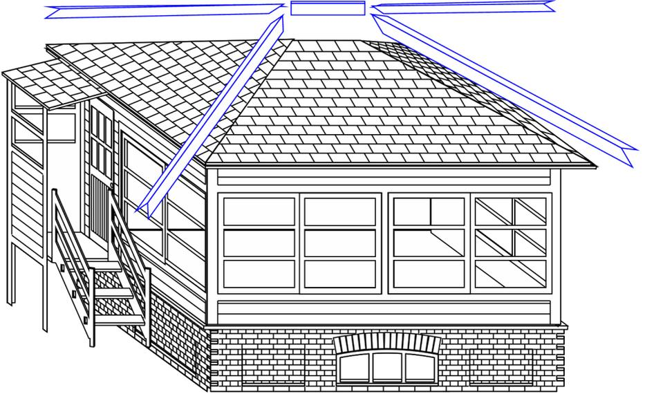
Finish the signal box by cutting the ridge tiles to size. Bend the ridge tiles along the middle score line, offer them to the roof and trim away parts that are protruding.
