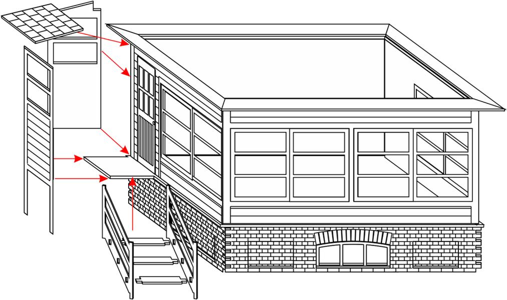
Cut out the two main elements for the porch from the “FLOOR” spruce. The back element with one leg should be glued flush to the back panel of the cabin. It should also index with the roof ledge. Second, side, element should be glued so that it is flush with the rear porch element. Finish the porch with the roof tiles panel from “ROOF TILES” spruce. The tiles should push into the gap under the top, thinner, ledge element.
