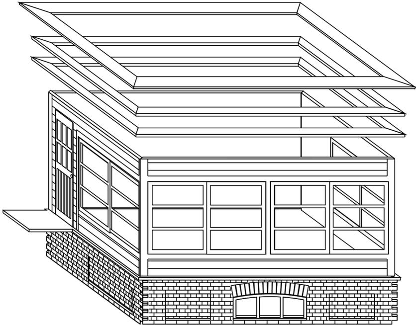
Start by using the thicker ledge elements from spruce labelled “ROOF TRUSS”. Lay the parts one by one rather than gluing them into layers. This will help align them better with the cabin. All elements should protrude on the front and be flush with the back edge of the panel. Dry fit the elements before gluing.
