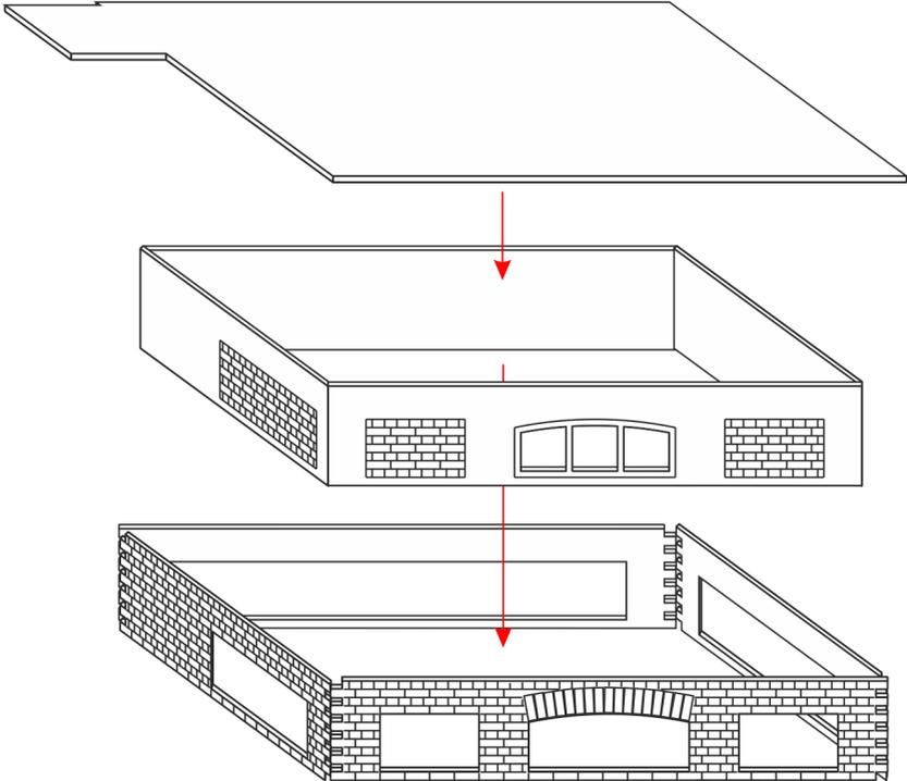
Glue windows and doors into the cabin panels. Shorter windows are for the front panel, wider windows for the side panels. Pay attention to the right side up of the front panel. Diagram below shows the corner overlap of the cabin sides.
