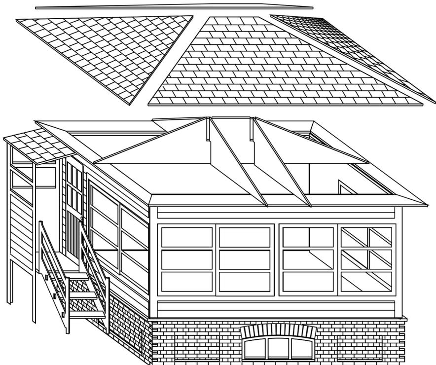
Start the roof assembly by gluing the trusses together. Glue the longer, front and back, roof tile panels to the truss assembly. Align the top edge of the panel with the top of the truss. Glue the side tile panels to the roof assembly in between the gaps. We recommend to glue the roof on a flat surface. The material used is flexible and can be bent a little if the roof doesn't turnout completely flat.
