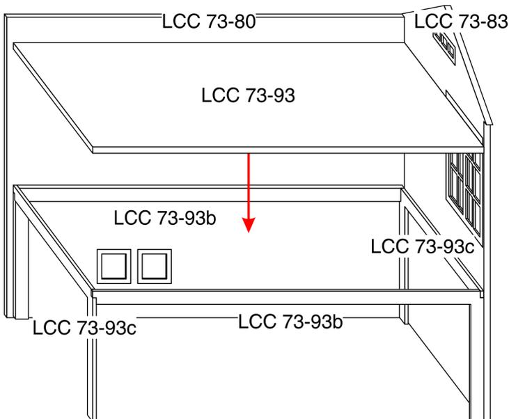
Start the main assembly by joining either the front or the back wall to one of the side walls. Use the floor to strengthen the walls as well as keep them square to each other. Make sure that the back and front walls are overlapping the side walls (the notches near gable on side walls should not be sticking out but be over the front or back wall).
