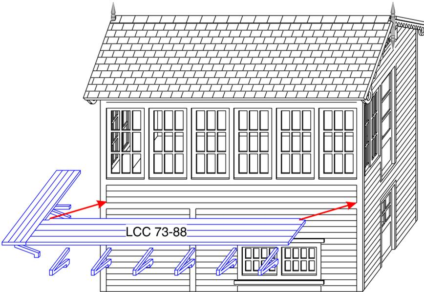
The balcony can be assembled either in the full version or in the front wall version only. Glue the supports from LCC 73-88 to the bottom of the balconies. Mind the cut outs in the balcony so that it clears the raised woodwork and sits flush on the signal box front wall. Glue the balcony to the signal box one plank below the windows (the supports should clear the raised woodwork).
