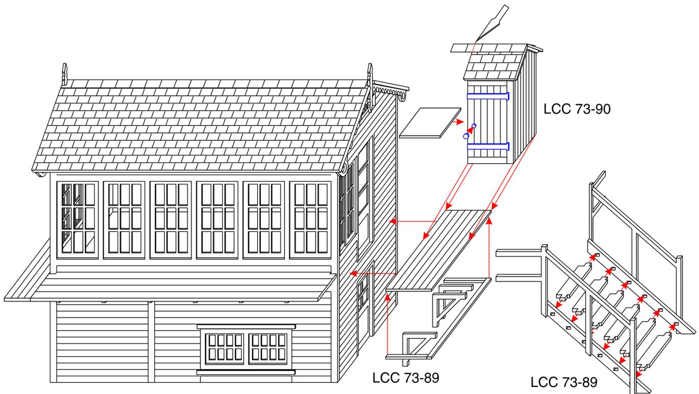
Diagram above shows the assembly of the stairs, stair balcony, and the priv.
