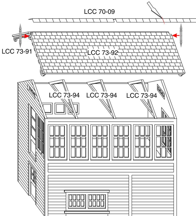
If assembling the roof separate (removable) glue the LCC 73-94 supports to the roof tile panels LCC 73-92. Otherwise glue them to the signal box body. The barge boards LCC 73-91 should be glued to the roof tile panels about flush with the cut out in the top edge of the roof tile panel. They also should not be touching the signal box body. Use the provided LCC 70-09 roof tile strips to complete the roof.
