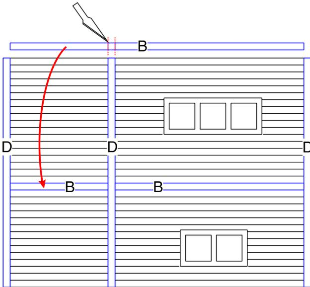
Use the 3 diagrams above to position the raised woodwork elements over the signal box front and back elevations. Note the element B needs to be cut along the scored lines to fit in place.
