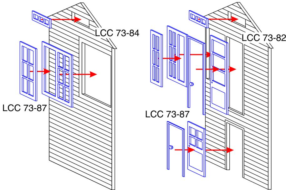
Use the diagrams on previous and this page to mount the windows and doors in the signal box. Pay attention to how the windows on side elevations are positioned. The sliding, top, windows should be facing the rear of the signal box.
