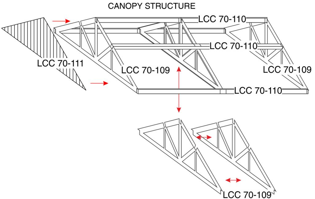
Start by gluing two LCC 70-109 together. Glue LCC 70-111 to one of the single LCC 70-109 elements. Ensure that the parts are flush with each other at the top. Using LCC 70-110 strips glue LCC 70-109 together to form the internal structure of the canopy. Use the markings in the middle of LCC 70-110 to align the doubled up LCC 70-109. Because LCC 70-110 have been shortened only on one side make sure LCC 70-110 are facing in the same direction to ensure correct alignment.
