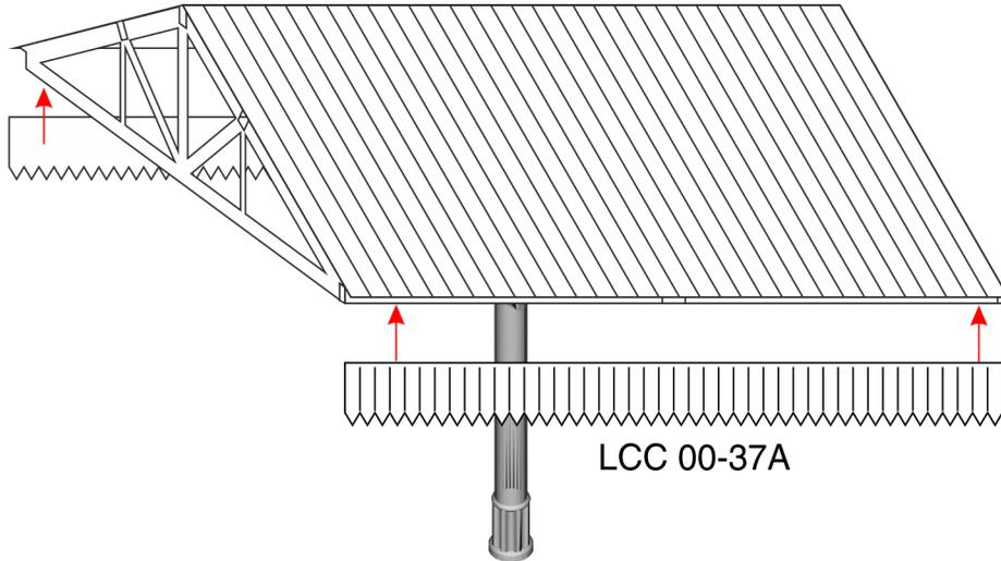
Last step is to glue the valence (LCC 00-37A) to the sides of the canopy section.
