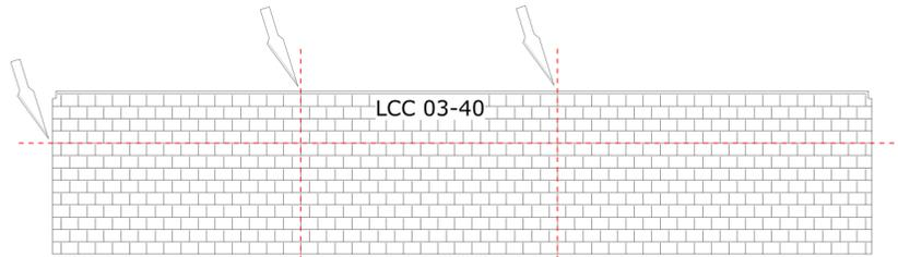
Cut out roof pieces from LCC 03-40 to fit the structure.
