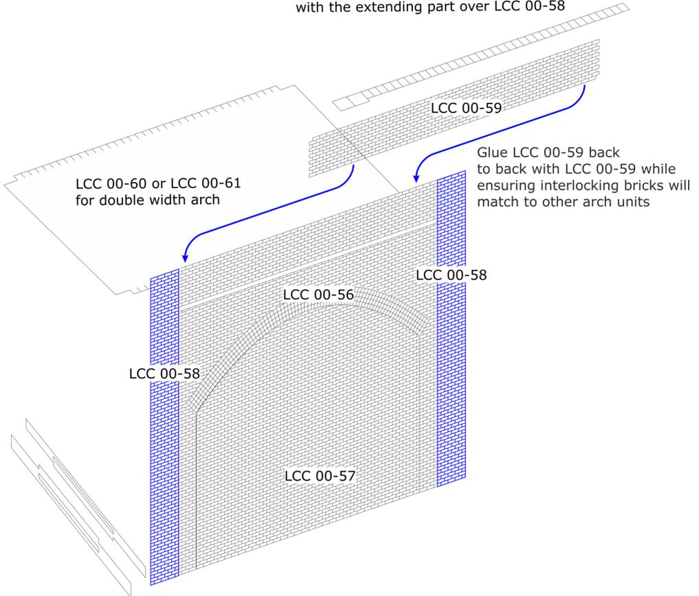
Glue LCC 00-59 back to back with LCC 00-59 while ensuring interlocking bricks will match to other arch units
